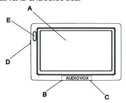
Figure 1. LCM45NB Monitor Controls and Indicators
